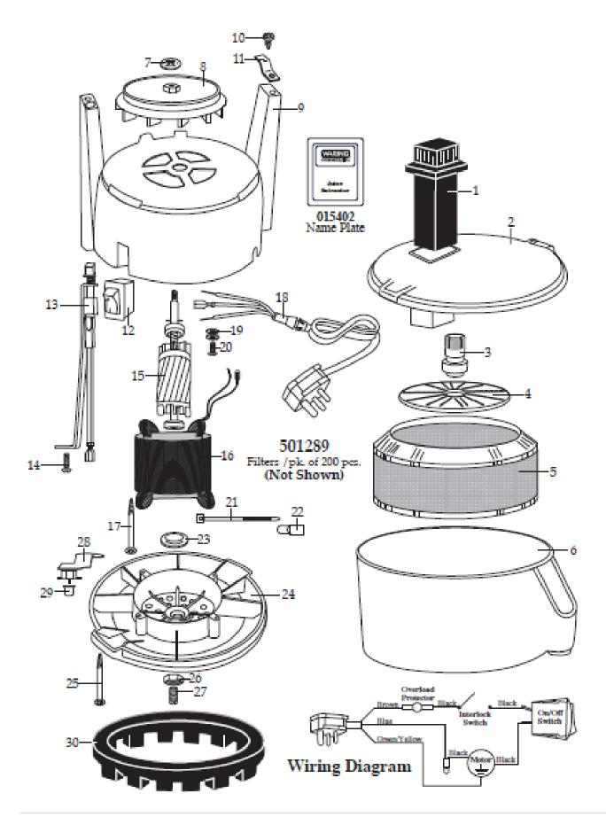
Exploded diagram and spare parts list CE380 & K199
