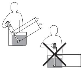
• For maximum efficiency we suggest to hold the mixer in an oblique position without placing the blade protector on the bottom of the cooking-pot.
