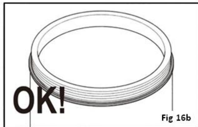
Moisten the gasket seal with water and fit the bowl back into place.
